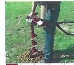
7 For safety, always keep leg pad against leg while digging.
